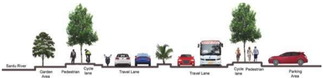
Figure 5-6 Typical section of river corridor
